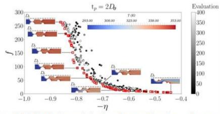
Figure 1: Multiobjective optimisation of a cross-flow heat exchanger using Bayesian methods[1]
